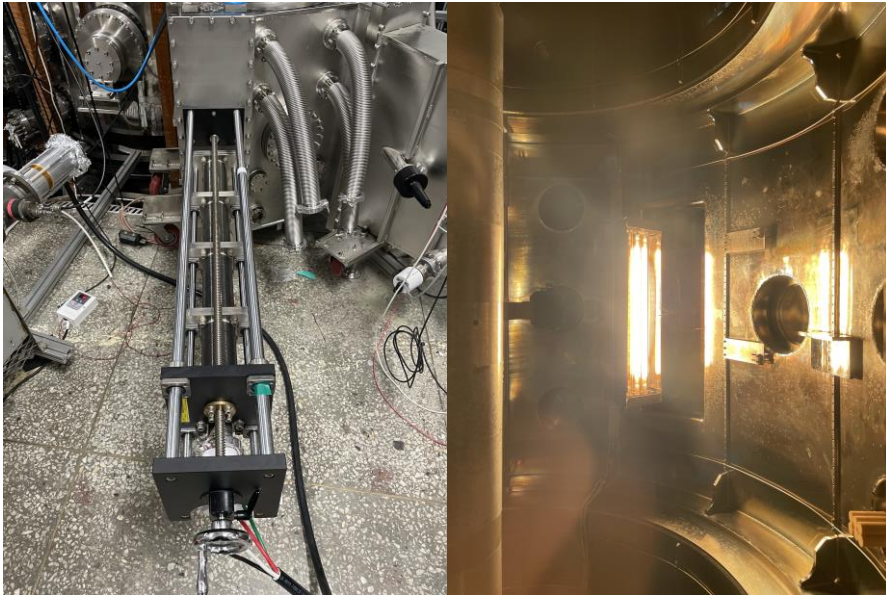
Fig 5. Movable halogen lamp for the center stack and the local outer mid plane wall baking
