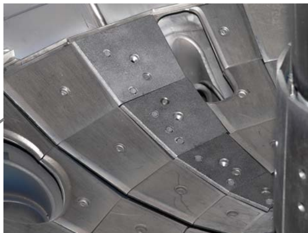
Array of 10 Langmuir probes in the divertor area
